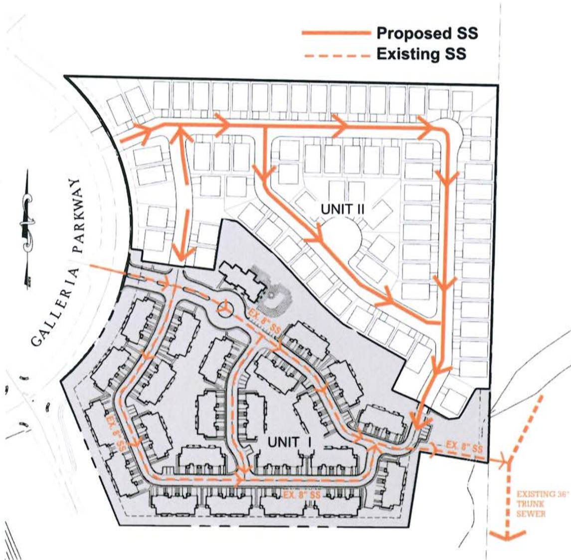
Figure 11 Phase II - Sanitary Sewer Improvements
